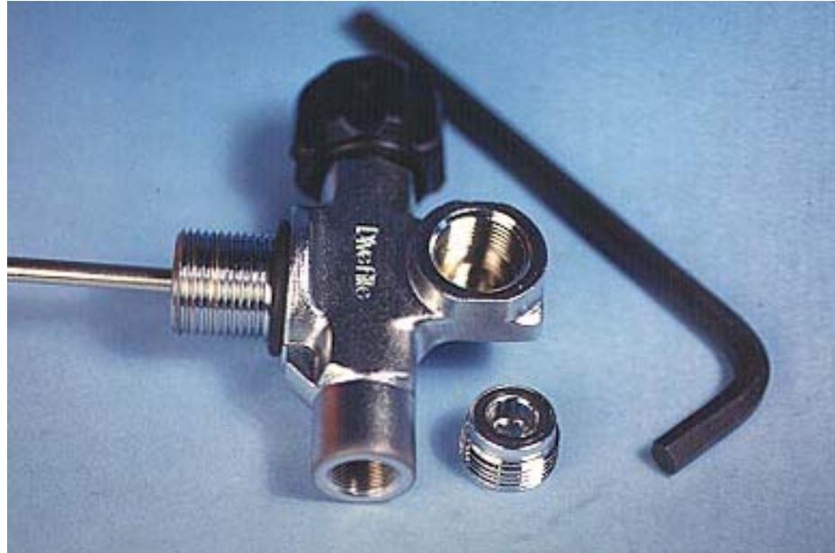
**Remove the DIN Adapter using a 8mm hex wrench**
