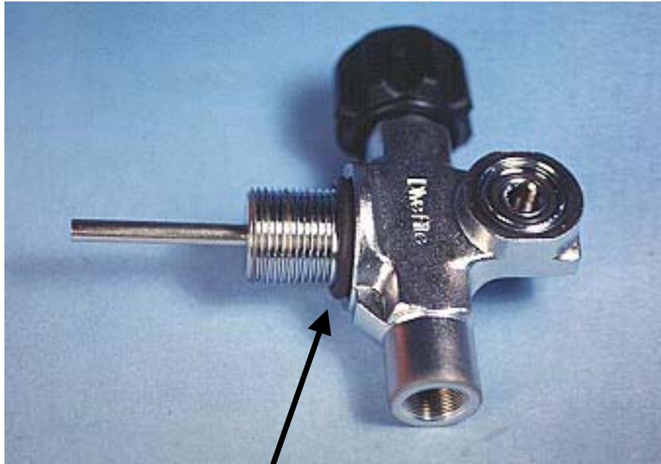
**Lubricate and Install “O” ring Part # VA2556**
