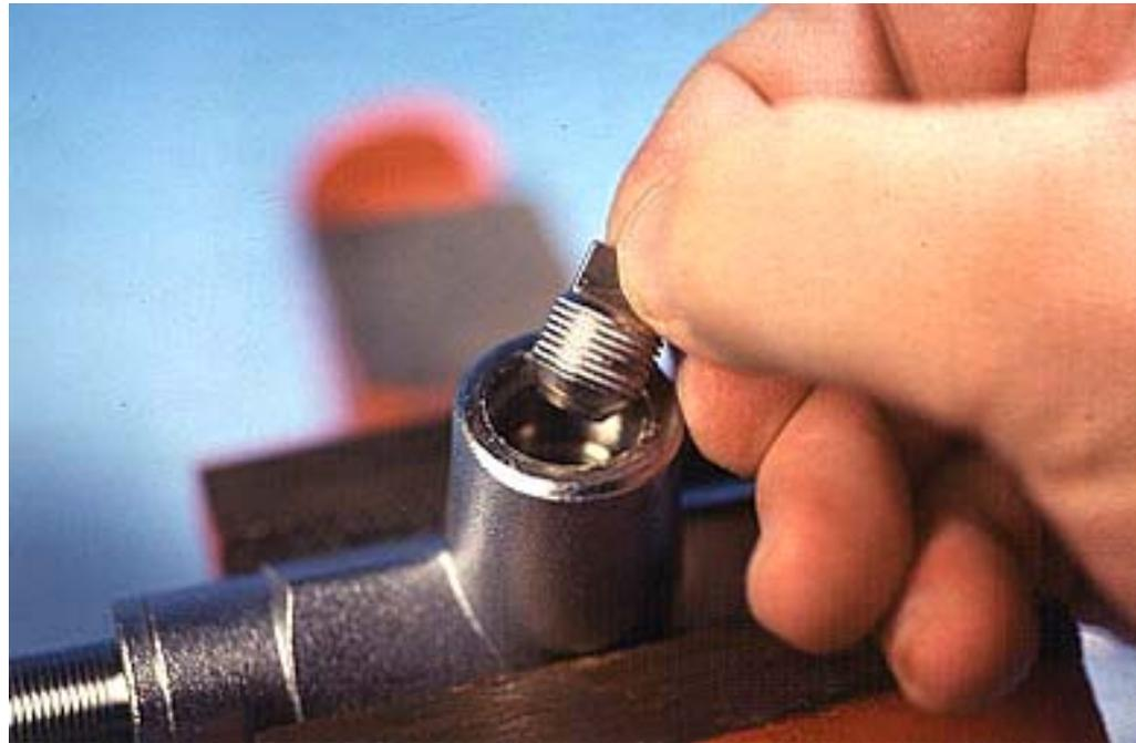
**Lubricate and install “O” ring VA2553 first,
