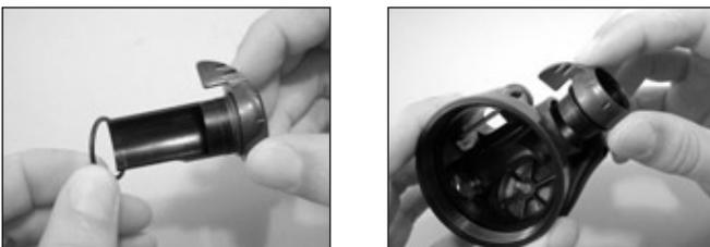
12. While depressing the lever, insert the valve body through the venturi lever and into the box bottom. Be sure that the two index flats and the two lever feet engage the tabs molded into the box bottom.
