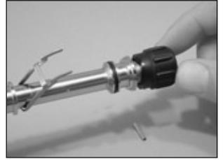
9. Unscrew the adjustment knob (34) and completely remove it from the valve body. Tilt the knob so the adjustment pin (31) falls out.
