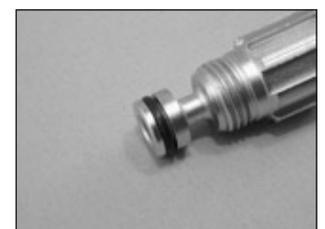
8. Install a new, lubricated o-ring (35) onto the adjustment screw (36). Using a 4mm hex wrench, thread the adjustment screw into the adjustment knob (33) until it stops. Preadjust the adjustment screw as follows:
