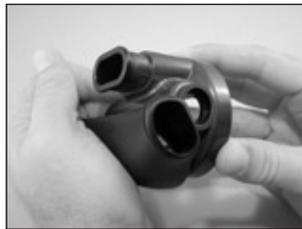
3. Install a new, lubricated o-ring (28) onto the stem of the shuttle valve (27). Press a new low pressure seat (26) into the front of the shuttle valve.
