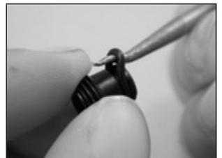
12. Remove the o-ring (22) from the valve body.
