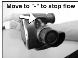
22. Turn off the air supply and purge the second-stage by pressing on the lever. Pull back on the adjustment wheel and unscrew the inline tool from the second-stage. Remove the hose from the inline tool.
