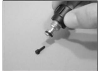
10. Remove the o-ring (32) from the adjustment knob. Using the LX tool (pn 129001), unscrew the plug (37). Remove the grip (34) by pulling it straight off the adjustment knob.
