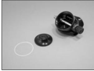
5. Using an  $\frac{1}{16}$ " wrench, unscrew the retaining nut (15). Remove the heat exchanger (16).
