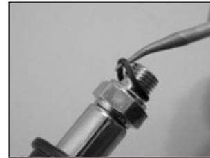
2. Pull back the two hose protectors (39 & 41) and inspect the hose crimps. The crimps should be free from damage and the hose should not be pulling out of the crimp. If it is, the hose must be replaced.
