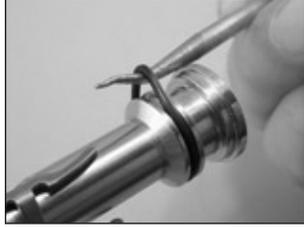
13. Insert a small 1/8" wooden dowel into the threaded end of the valve body and push out the shuttle valve assembly (26-30). Separate the shuttle valve assembly by pulling on each end.
