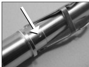
6. With the “feet” of the shuttle valve pointing downward (away from the lever) and the lever pointing straight up (perpendicular to the valve body), insert the valve assembly into the valve body. Using your finger, press the shuttle valve assembly all the way into the valve body, pass the lever feet. To make sure the shuttle valve assembly is installed correctly, hold the valve body by the threaded end. The shuttle valve should stay in the valve body.
