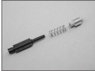
14. Using a fingernail, remove the LP seat (26) and small o-ring (28) from the shuttle valve.
