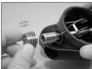
6. Turn the adjustment knob counterclockwise until it stops. Press the lever (25) against the valve body (23). While keeping the lever depressed, grasp the knob and pull the valve body assembly out of the box bottom (9). Remove the valve body o-ring (17) that will probably be left behind in the left side of the box bottom as you look at it.
