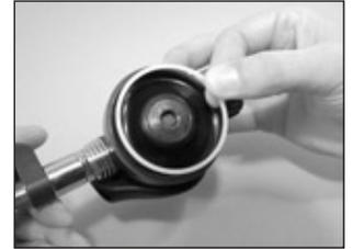
19. Screw in the diaphragm retainer (5), flat side facing the diaphragm, until fingertight. Use the Titan LX diaphragm retaining tool (p/n 129001) to tighten approximately another ¼ turn. After installing the diaphragm
