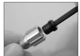
9. Press the grip (34) onto the adjustment knob. Using the LX Tool, screw the plug (37) into the end of the adjustment knob.
