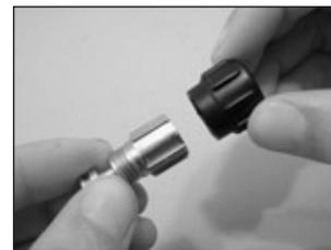
11. Using a 4mm hex wrench, remove the adjustment screw (36). Remove the o-ring (35) from the adjustment screw.
