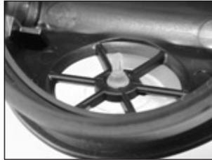
2. Soak the exhaust tee in hot water (~125°F) for 2 to 3 minutes. Install the exhaust tee (14) onto the flange on the outside of the box bottom. Begin by hanging the exhaust tee on the top of the flange, then press the bottom of the tee into place.
