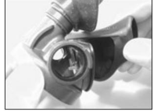
17. Fold back the edges of the exhaust valve (13) and inspect underneath. The seating surface should be clean and free of damage. Inspect the exhaust valve. It should be supple and have well defined edges. If it looks good, there is no need to remove it and it may be reused. If there is any sign of deterioration, it should be replaced.
