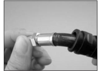
3. Using your hand, unscrew the retaining ring (1). Separate the retaining ring from the rubber mating ring (2). Lift out the purge cover (4).
