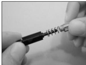
5. If you removed the lever, replace it so that the lever is on the same side as the small dimple on the valve body and the outlet port is pointing to the right as the threaded inlet side faces away from you.
