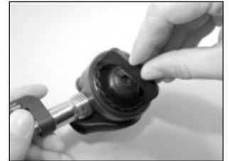
retainer, grab the edges of the strike plate and gently tug the diaphragm to the left, right, top and bottom to make sure it is secure in the box bottom. If the diaphragm pulls out, then you need to reinstall it.
