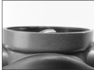
16. Add a new o-ring (42) to the male end of the medium pressure hose. Install a new, lubricated o-ring (38) to the swivel end of the hose
